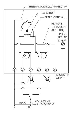
Actuator shown in open position Power to #1 & #2 To Open Power to #1 & #3 To Close
