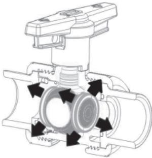
Since the seat is allowed to "float" in the open position, fluids and debris do not accumulate around and behind the seat. The result is a self-adjusting seat with reduced wear, smoother operation, and self cleaning action to keep the valve free of internal sediment and fluid stagnation.
