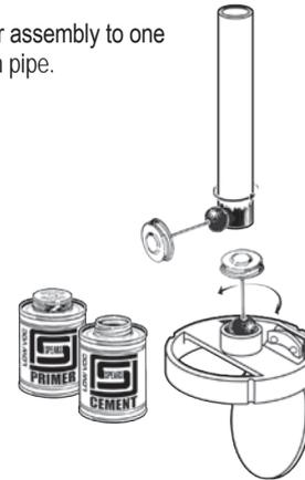
**STEP 6** Insert flapper assembly then install lid and tighten.
