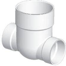
Utility Back Water Valve includes replaceable Flapper Assembly and requires use of an Extension Kit pressure rated to either 50 psi or 100 psi. Extension Kit includes 6" DWV Cleanout Adapter and a Threaded plug for use with user supplied 6" Schedule 40 or Class 125 Riser Extension Pipe cut to desired length. User supplied 1" or 1-1/4" coupling with 1-1/4" is used for the Internal Extension Pipe.
