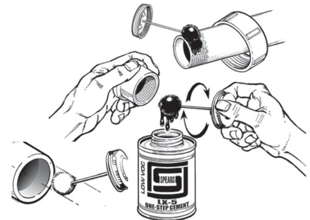
**STEP 3 Immediately Assemble Joint**
